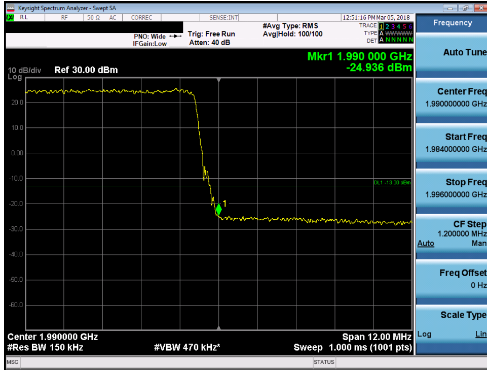
Plot 7-385. Upper Band Edge Plot (Band 2 - 15.0MHz 256-QAM)
