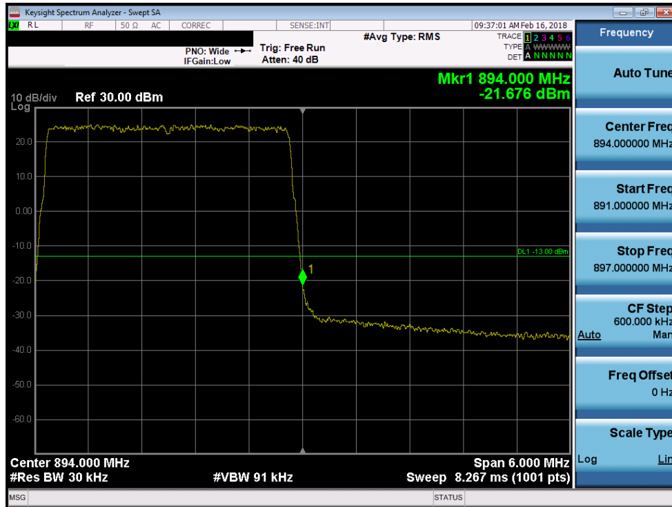
Plot 7-221. Upper Band Edge Plot (Band 5 - 3.0MHz 64-QAM)
