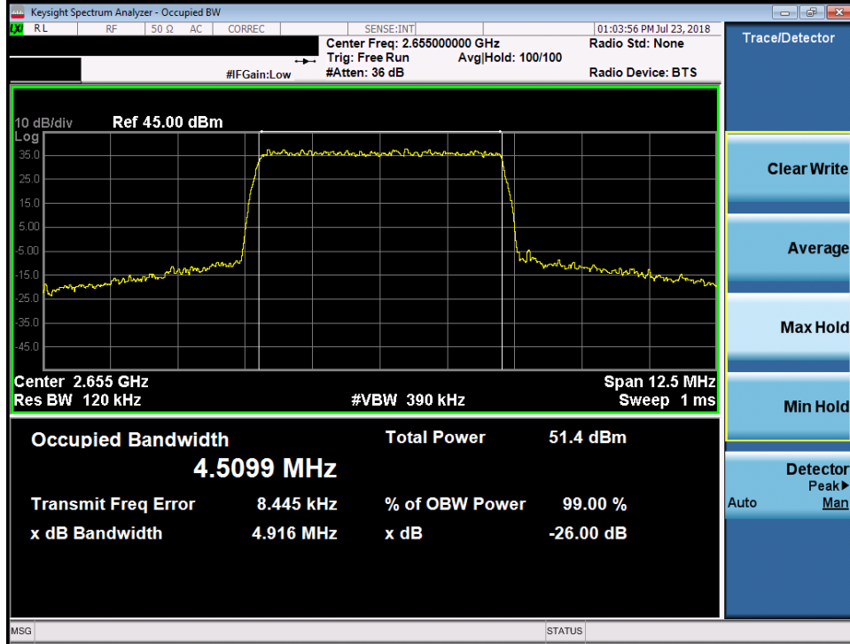
Plot 7-114. Occupied Bandwidth Plot (Band 7 - 5.0MHz 16-QAM)
