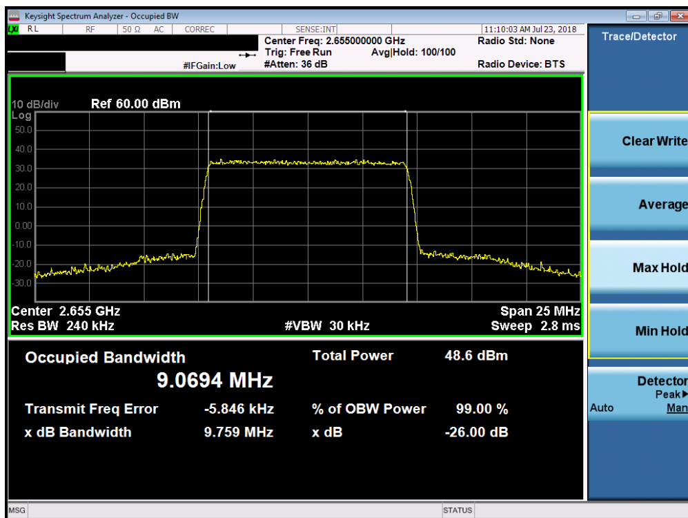
Plot 7-104. Occupied Bandwidth Plot (Band 7 - 10.0MHz 256-QAM)
