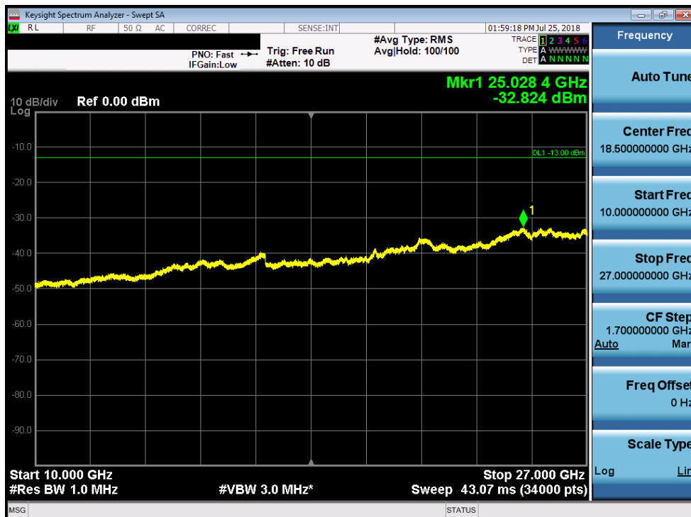
Plot 7-143. Conducted Spurious Plot (Band 7 - 10.0MHz QPSK – Mid Channel)
