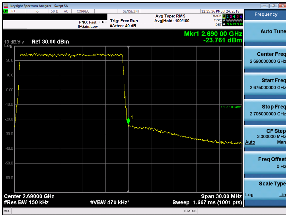
Plot 7-193. Upper Band Edge Plot (Band 7 - 15.0MHz 256-QAM)
