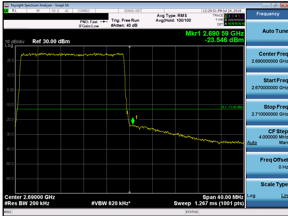
Plot 7-197. Upper Band Edge Plot (Band 7 - 20.0MHz QPSK)
