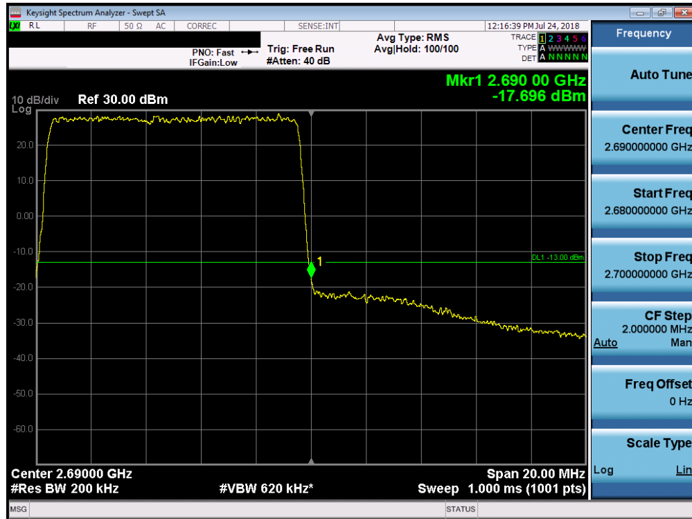
Plot 7-177. Upper Band Edge Plot (Band 7 - 10.0MHz 256-QAM)
