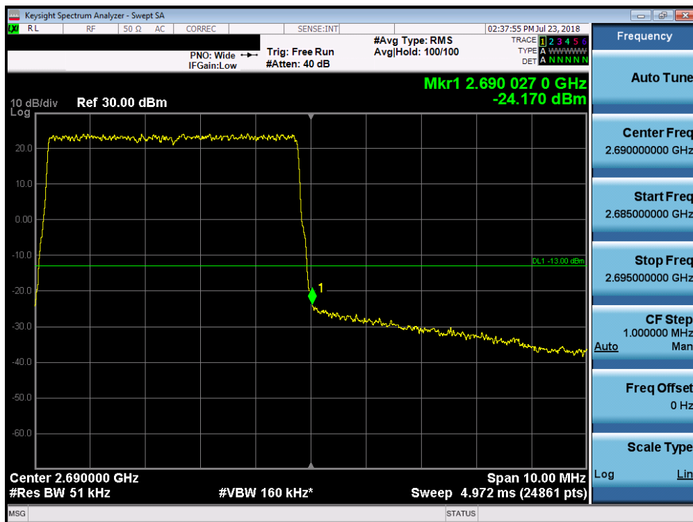
Plot 7-149. Upper Band Edge Plot (Band 7 - 5.0MHz QPSK)
