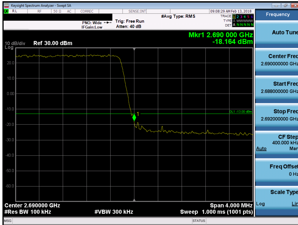
Plot 7-153. Upper Band Edge Plot (Band 41 - 5.0MHz 16-QAM)
