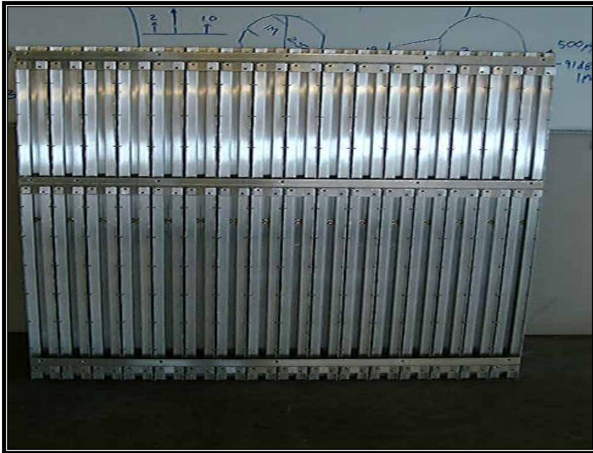
PHOTOGRAPH 10: BACK OF ANTENNA ARRAY
