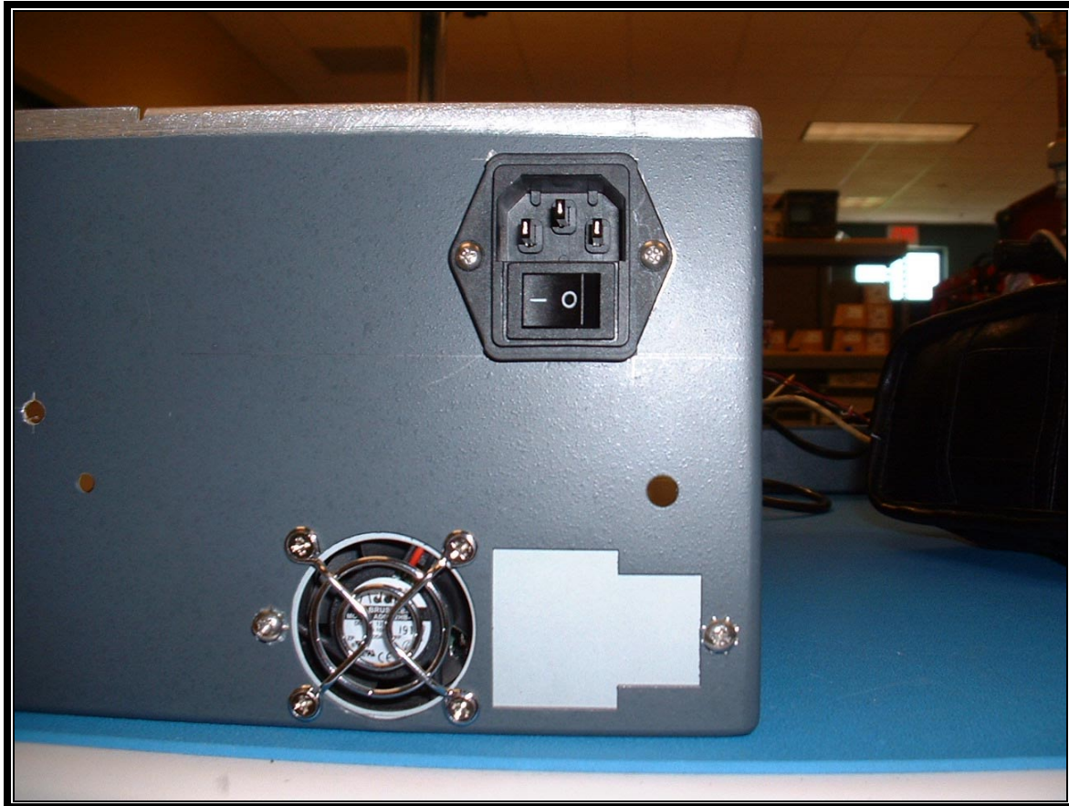
PHOTOGRAPH 17: AC LINE FILTER IMPLEMENTATION #3
