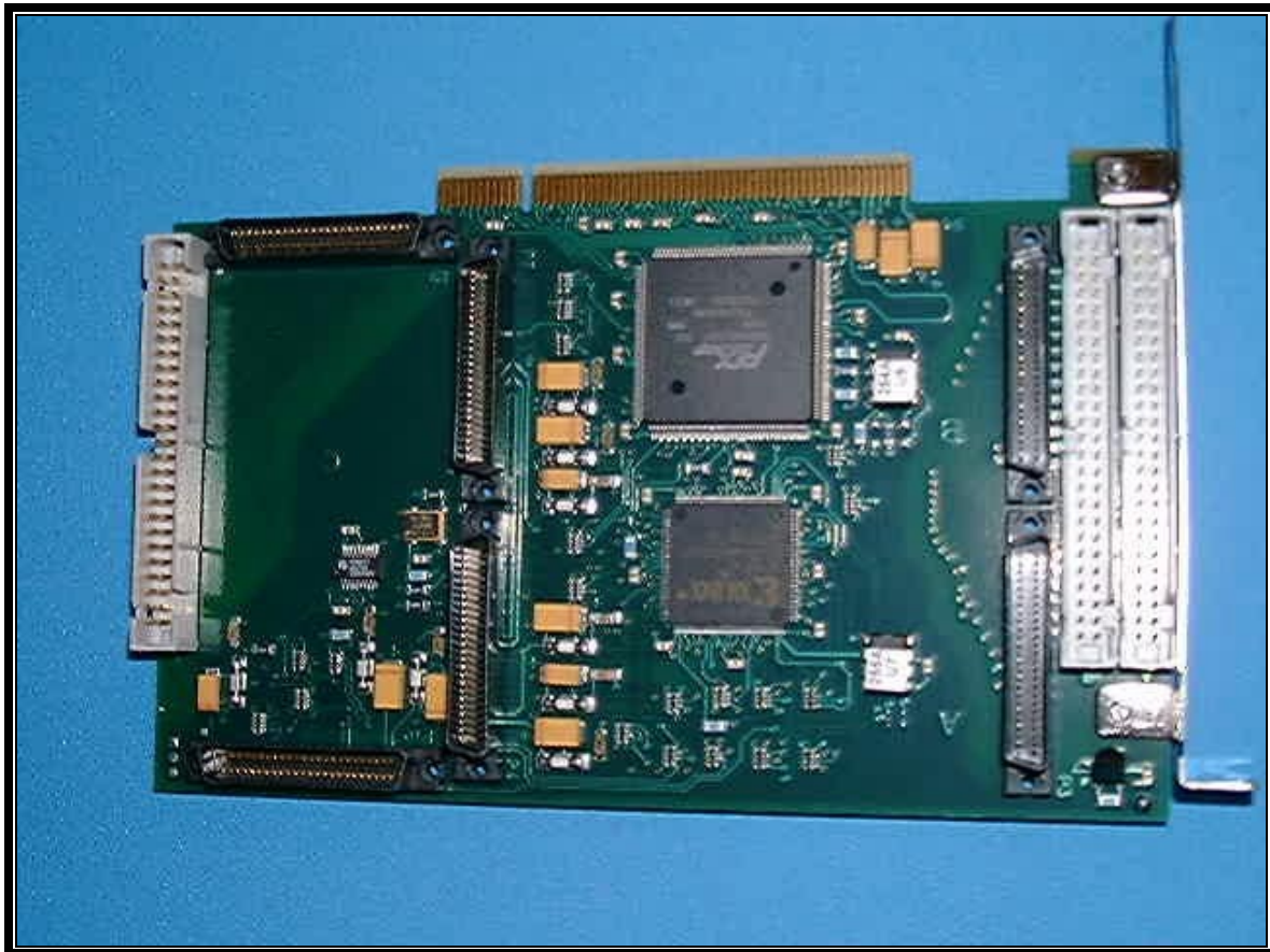
PHOTOGRAPH 33: DAC PCI CARRIER BOARD TOP
