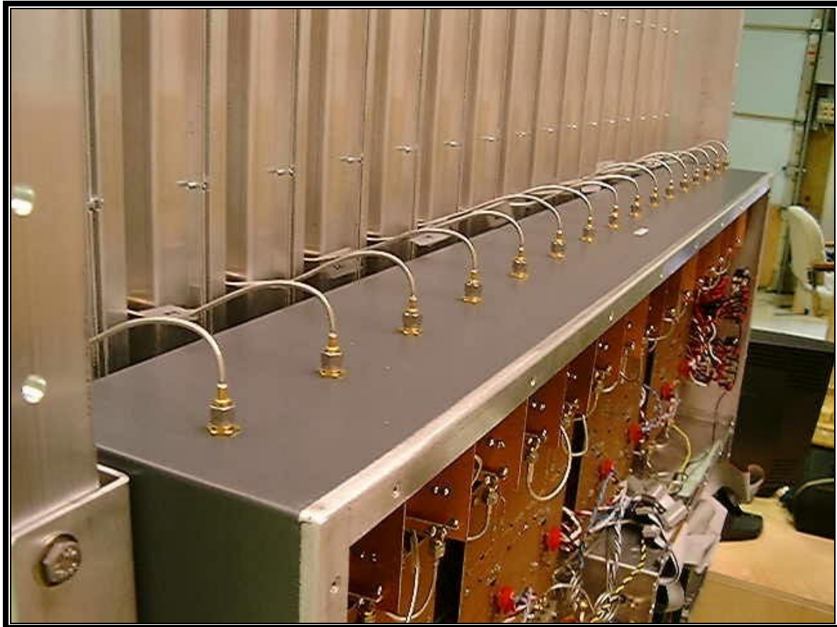
PHOTOGRAPH 54: RF PORT TO ANTENNA
