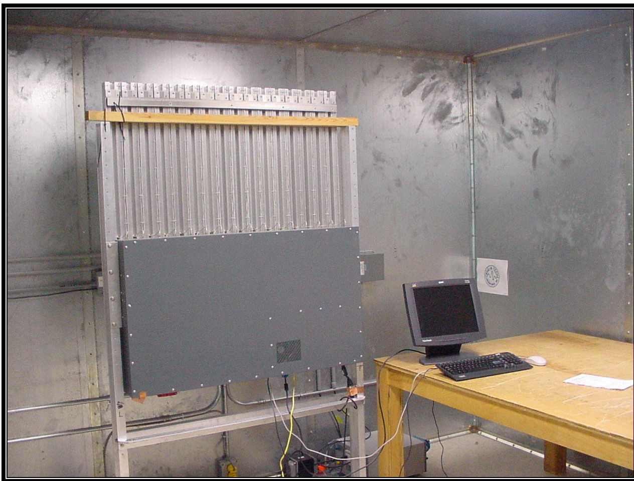
PHOTOGRAPH 6: CONDUCTED EMISSION REAR VIEW WORST-CASE CONFIGURATION
