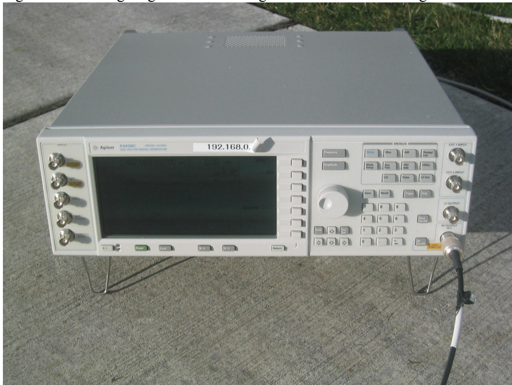
Figure 10: ESG Signal generator used to generate 2437GHz CW signal
