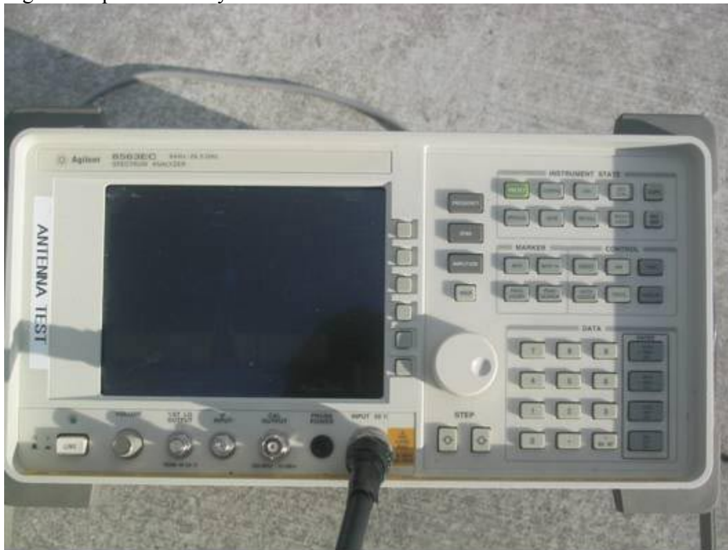
Figure 9: Spectrum analyzer used to make the measurement
