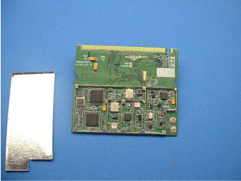
Figure 15 - Top of radio card - no shield
