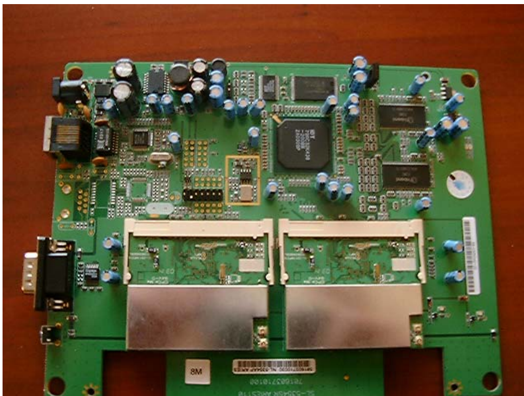
Figure 4 - Digital board with radios
