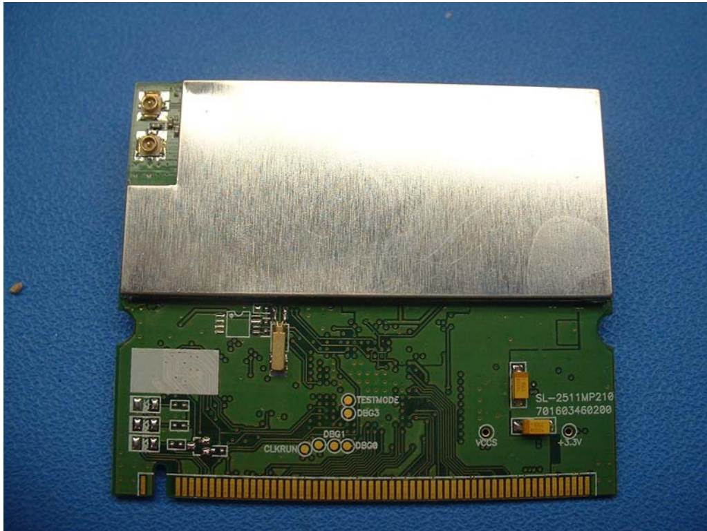
Figure 13 - Radio card top with shield
