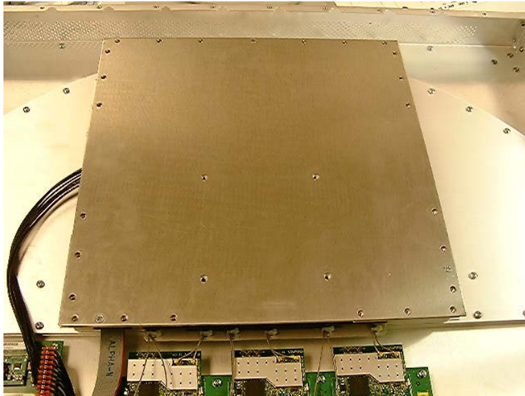
Figure 9 Plate over RF section
