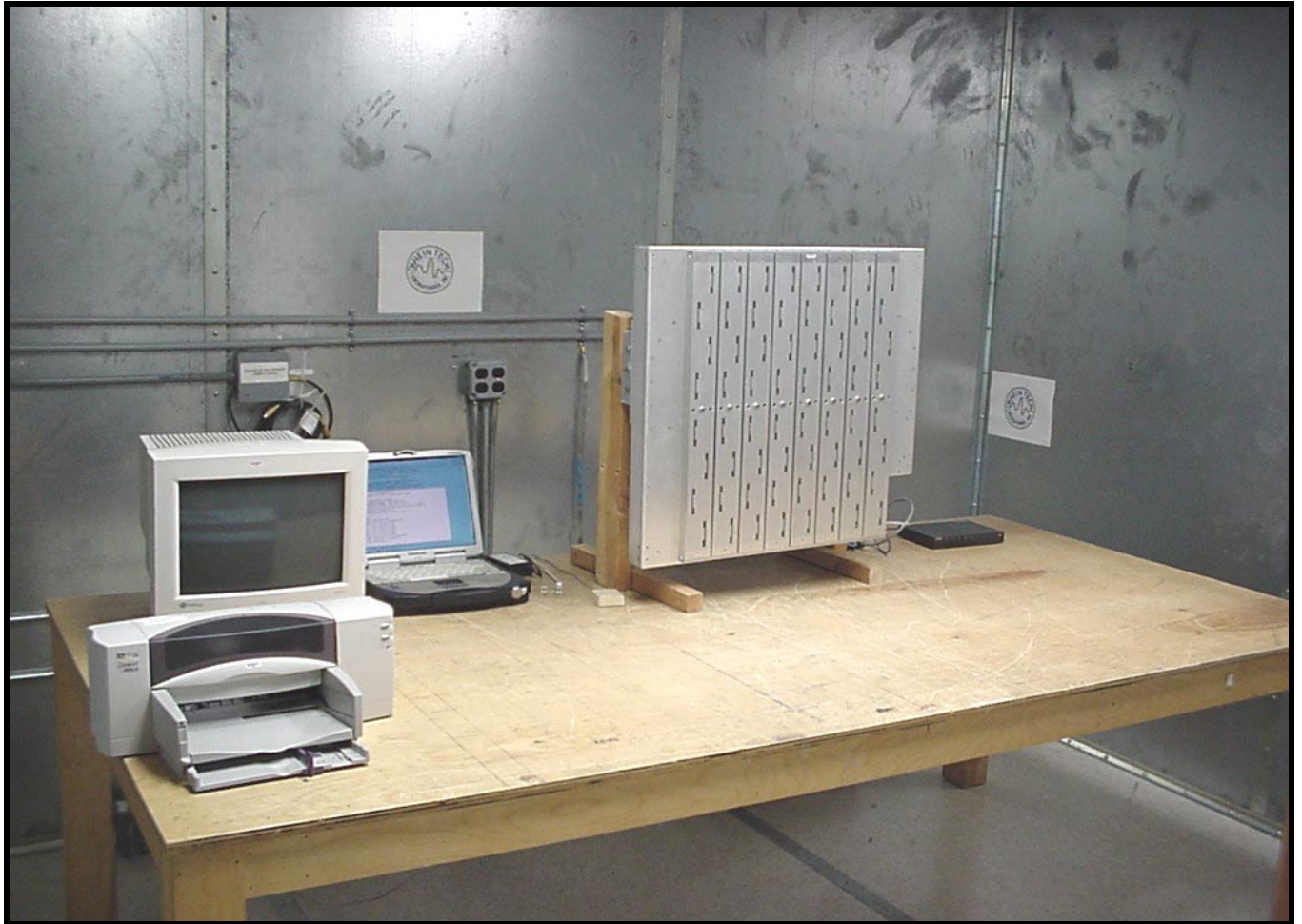
PHOTOGRAPH 1: AC CONDUCTED TEST FRONT VIEW
