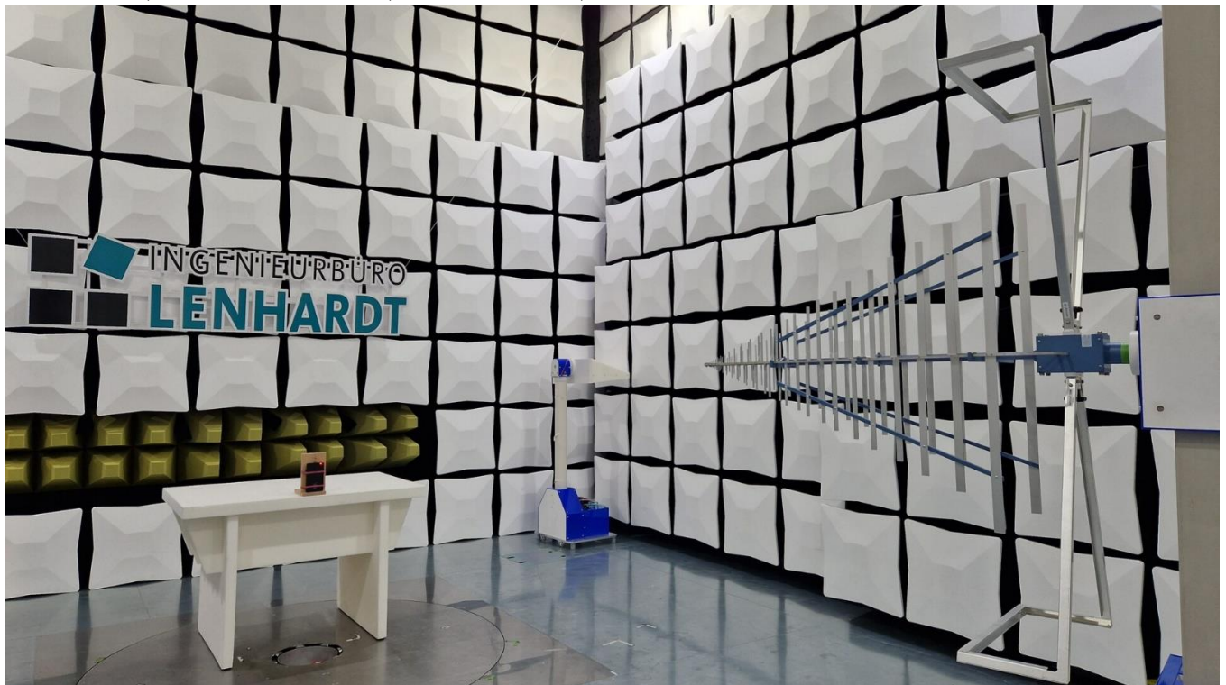
Photo No. 10, measurement in SAC, 30 MHz – 1 GHz, overall view:
