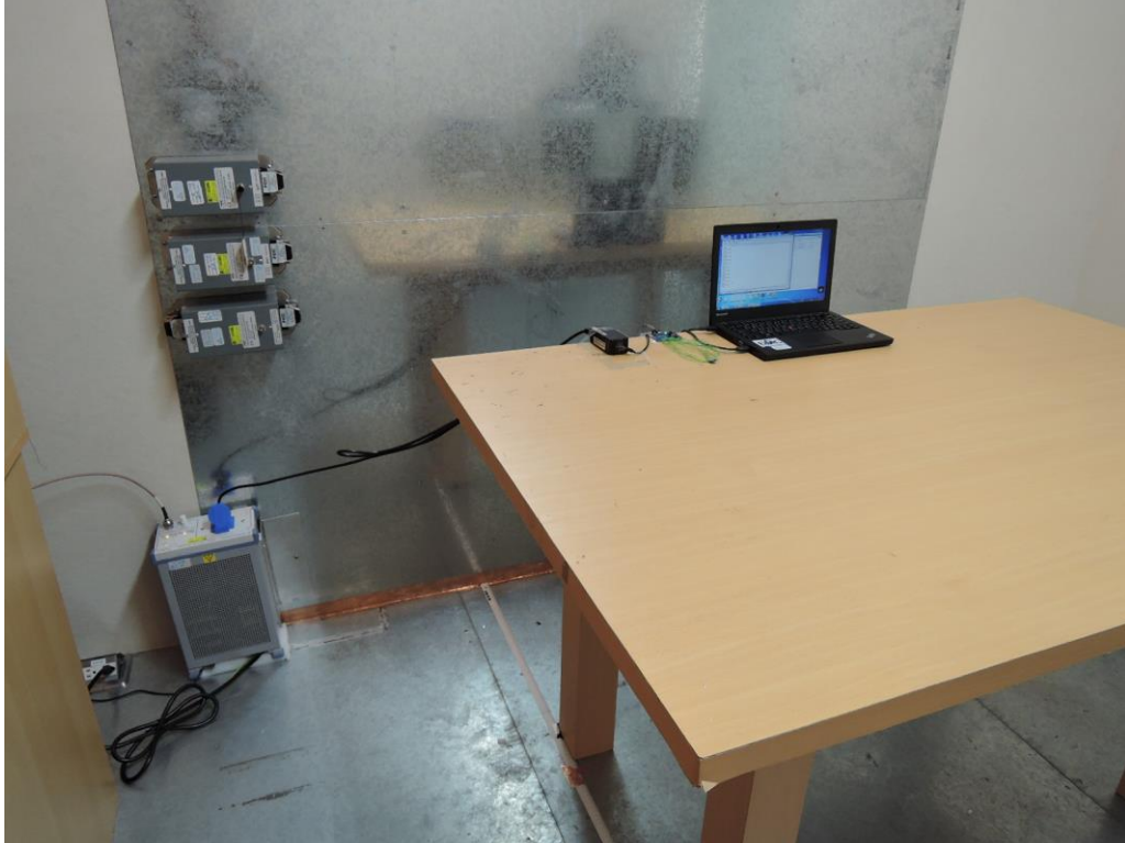
Photograph 6: Set-up for for Mains Conducted testing Front
