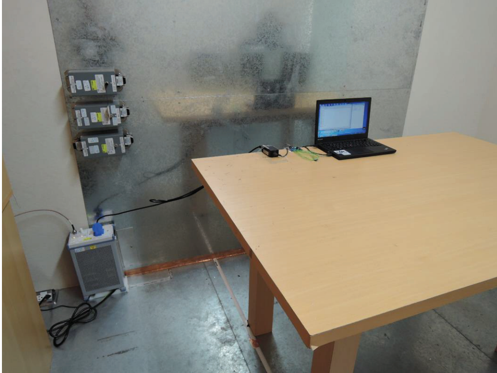
Photograph 6: Set-up for for Mains Conducted testing Front
