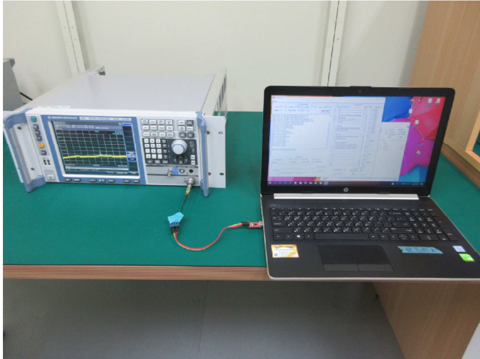
Photograph 5: Set-up for Conducted testing (View 1)
