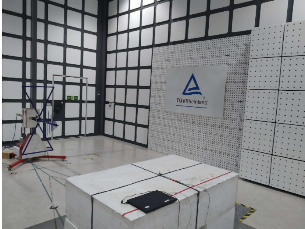
Photograph 3: Set-up for Spurious Emissions (Back View 1)
