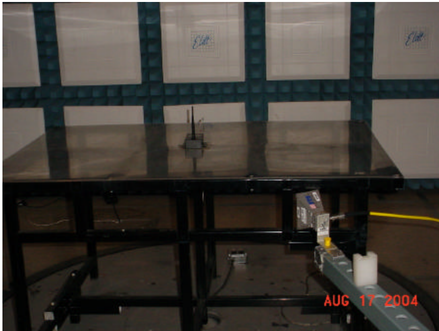
Test Setup for Radiated Emissions, 5GHz to 24GHz - Horizontal Polarization
