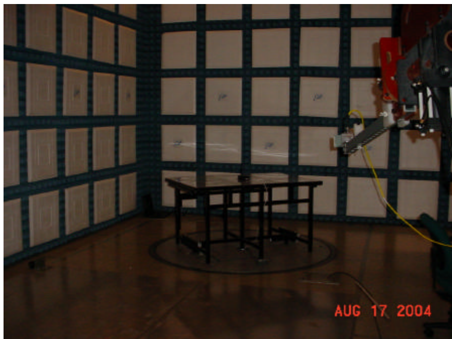
Test Setup for Radiated Emissions, 2GHz to 5GHz - Vertical Polarization
