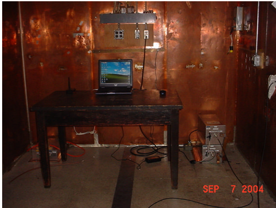
Test Setup for Conducted Emissions
