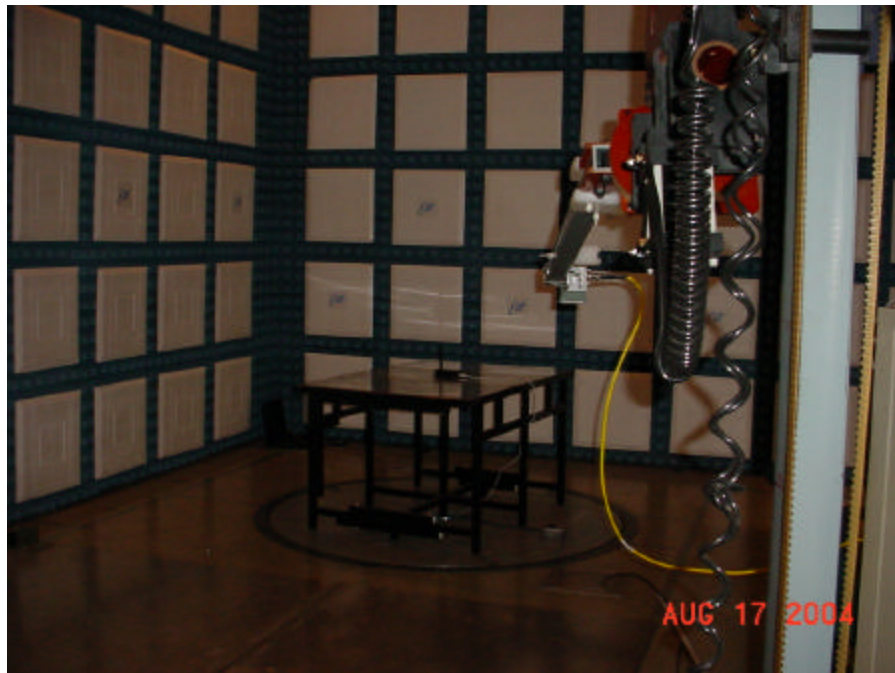
Test Setup for Radiated Emissions, 2GHz to 5GHz - Horizontal Polarization
