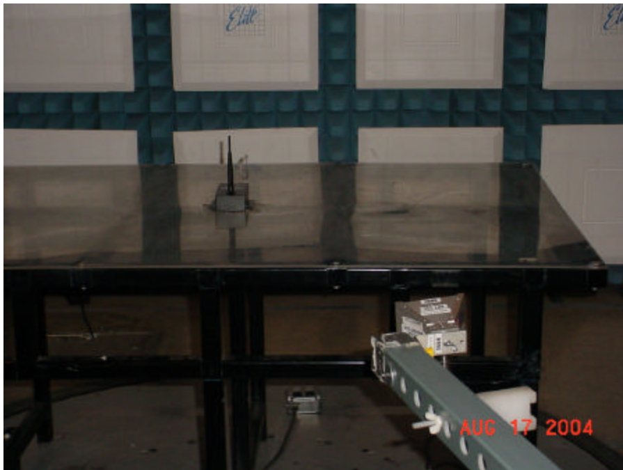
Test Setup for Radiated Emissions, 5GHz to 24GHz - Vertical Polarization
