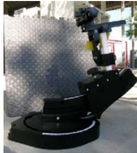
Device holder supplied by SPEAG
