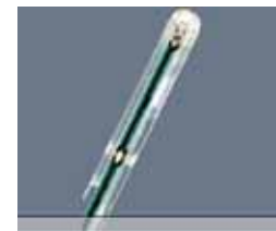
Figure 5 H-Field Free-space Probe
