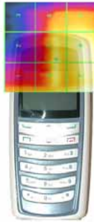
Figure 27 Sample E-field Scan Overlay
