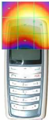
Figure 28 Sample H-field Scan Overlay
