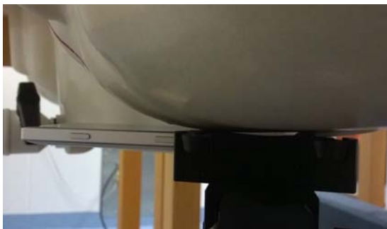
Photo of the Device in "cheek" position
