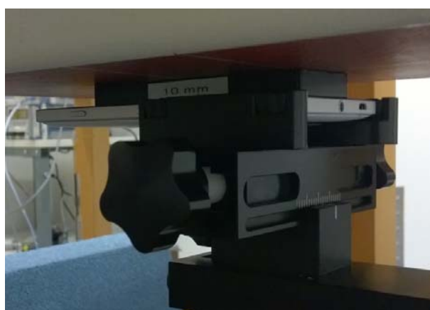
Photo of the device positioned for WR mode measurement – display facing phantom. The spacer was removed before the start of the measurements.
