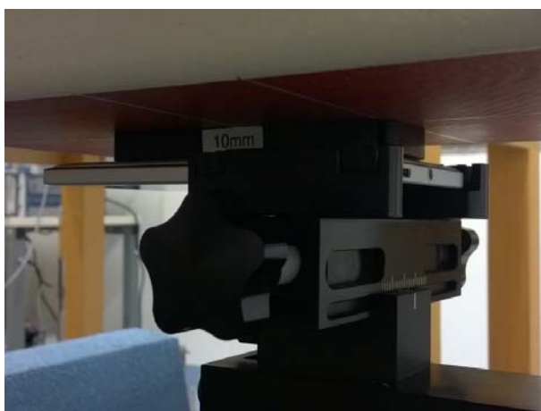
Photo of the device positioned for WR mode measurement –back facing phantom. The spacer was removed before the start of the measurements.
