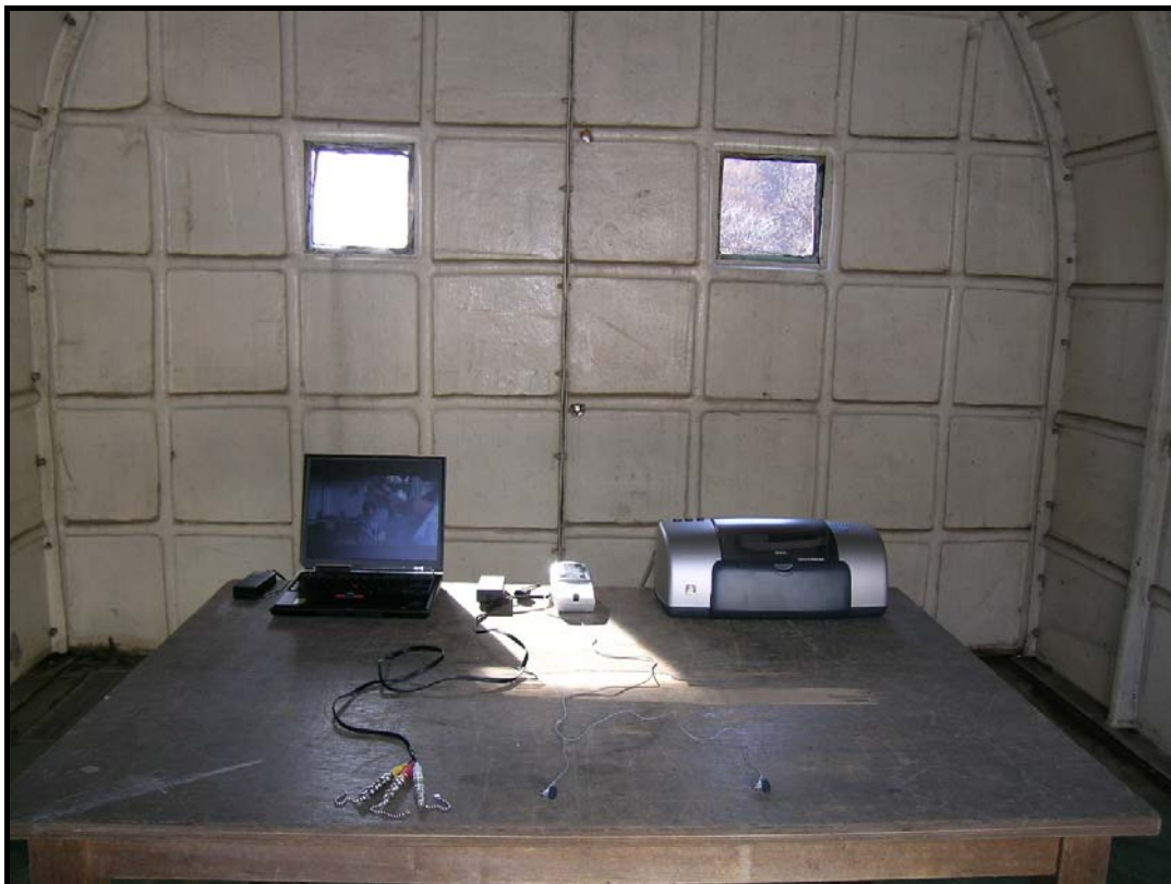
Photograph 2: Setup for Radiated Emissions
