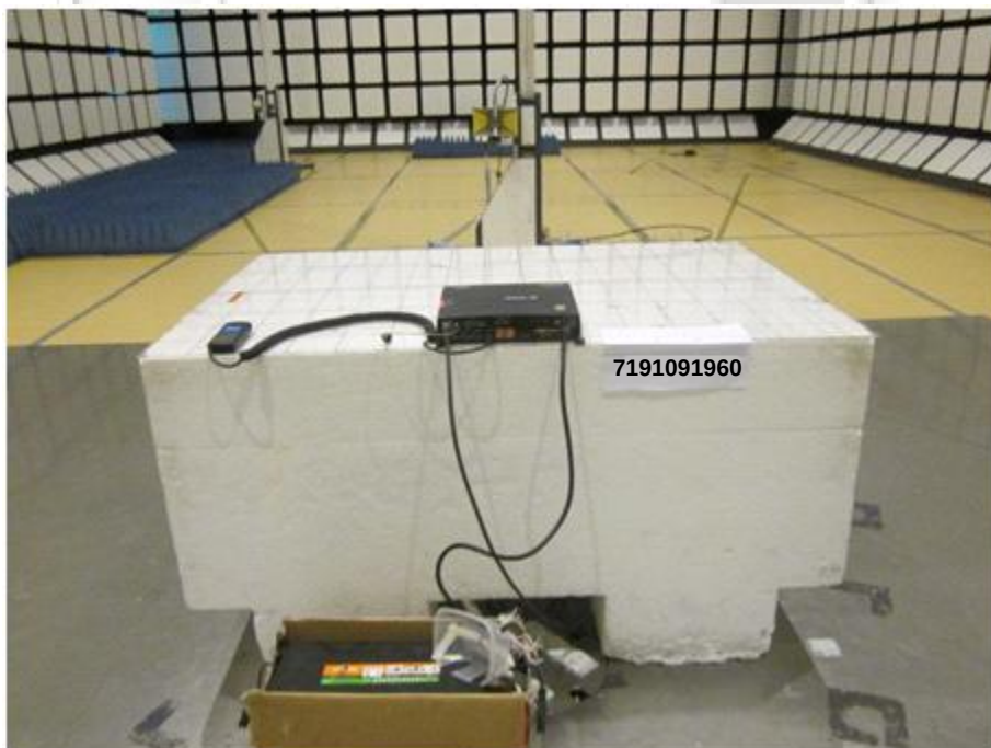
Band Edge Compliance (Radiated) Test Setup
