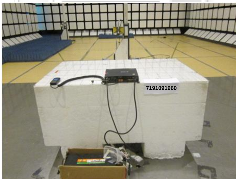
Radiated Emissions Test Setup (Rear View)
