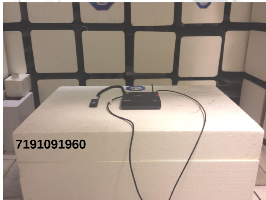
Radiated Spurious Emissions Test Setup (Rear View)
