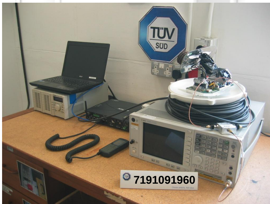
Unwanted Emissions at Antenna Terminal Test Setup
