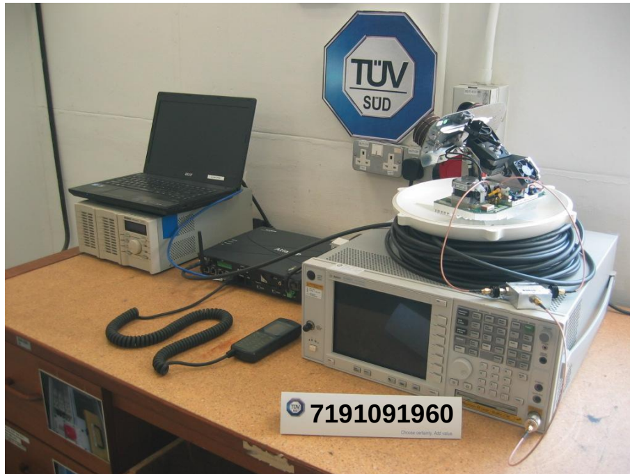
RF Output Power Test Setup
