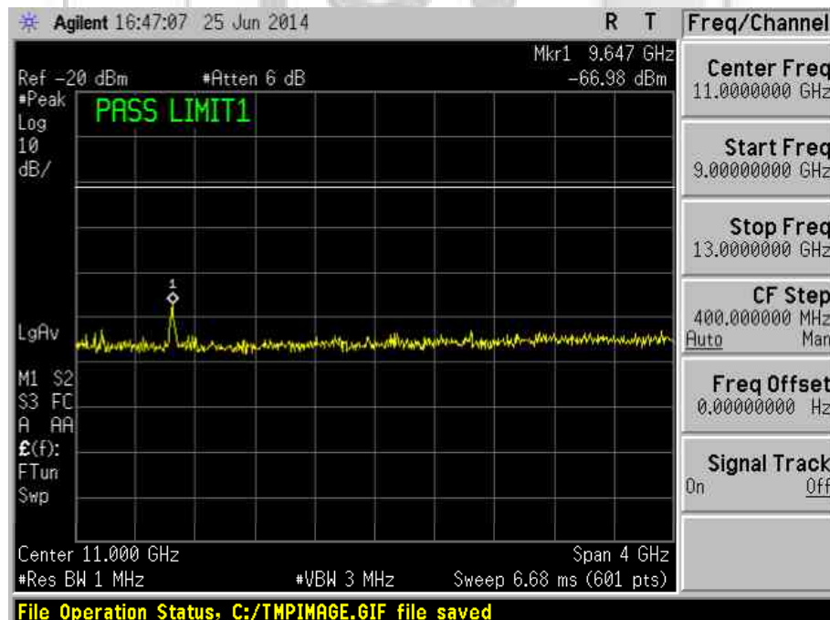
Plot 1581 – Channel 1 (lower ch) @ QPSK 18Mbps
