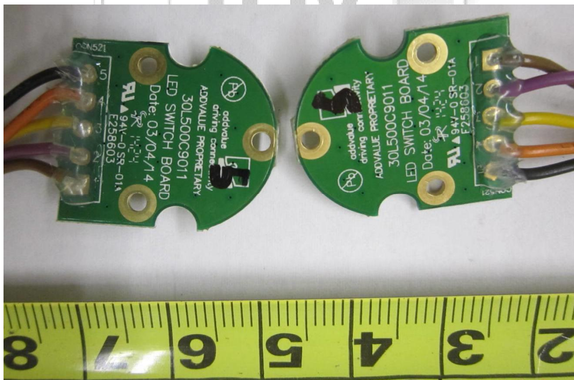
EUT Power ON/OFF Switch , Pointing Mode Switch PCB Trace Side
