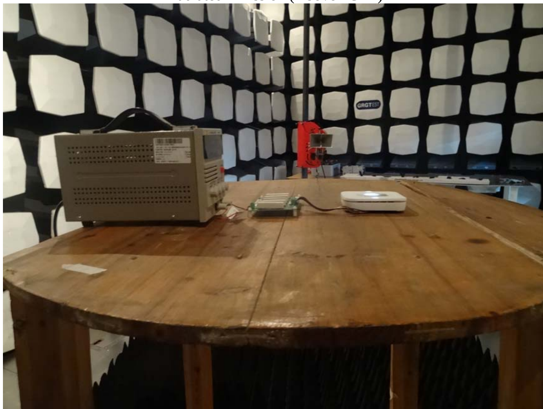
Radiated Emission (Above 1GHz)
