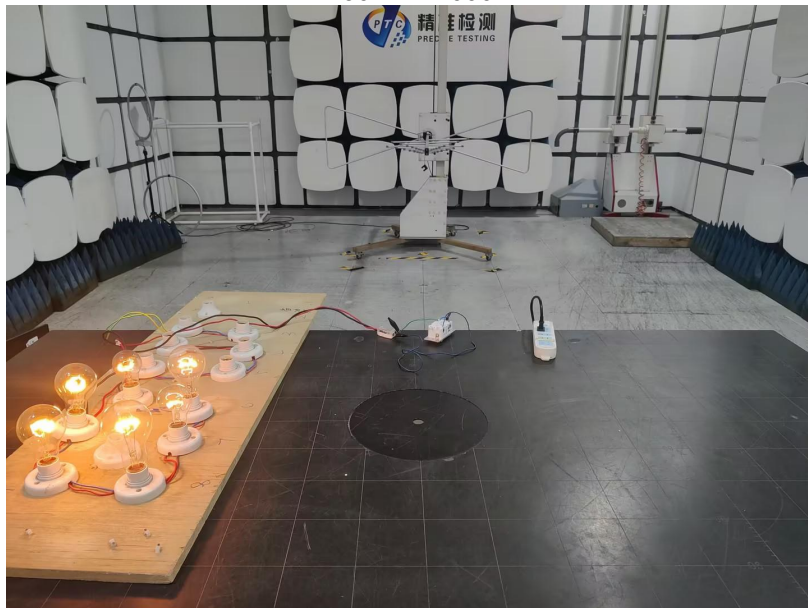
Radiated Spurious Emissions From 30MHz-1000MHz
