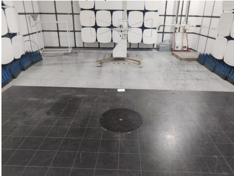
Radiated Spurious Emissions Test Frequency From 30MHz-1GHz
