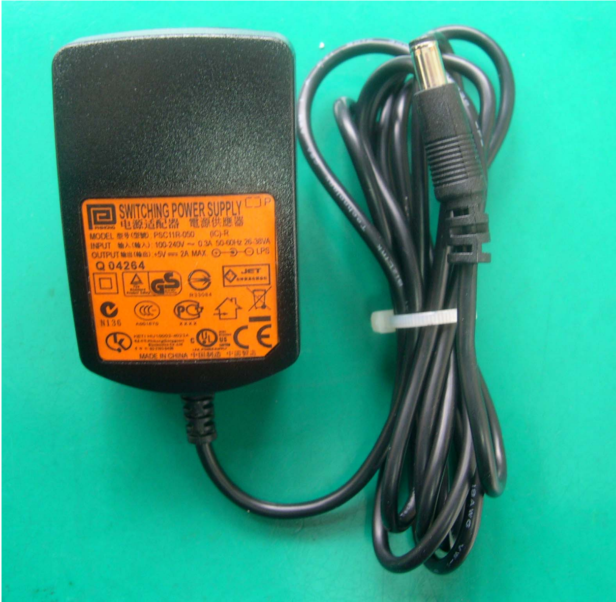
<Photograph 4: AC/DC Adaptor > For testing the power line conducted emissions
