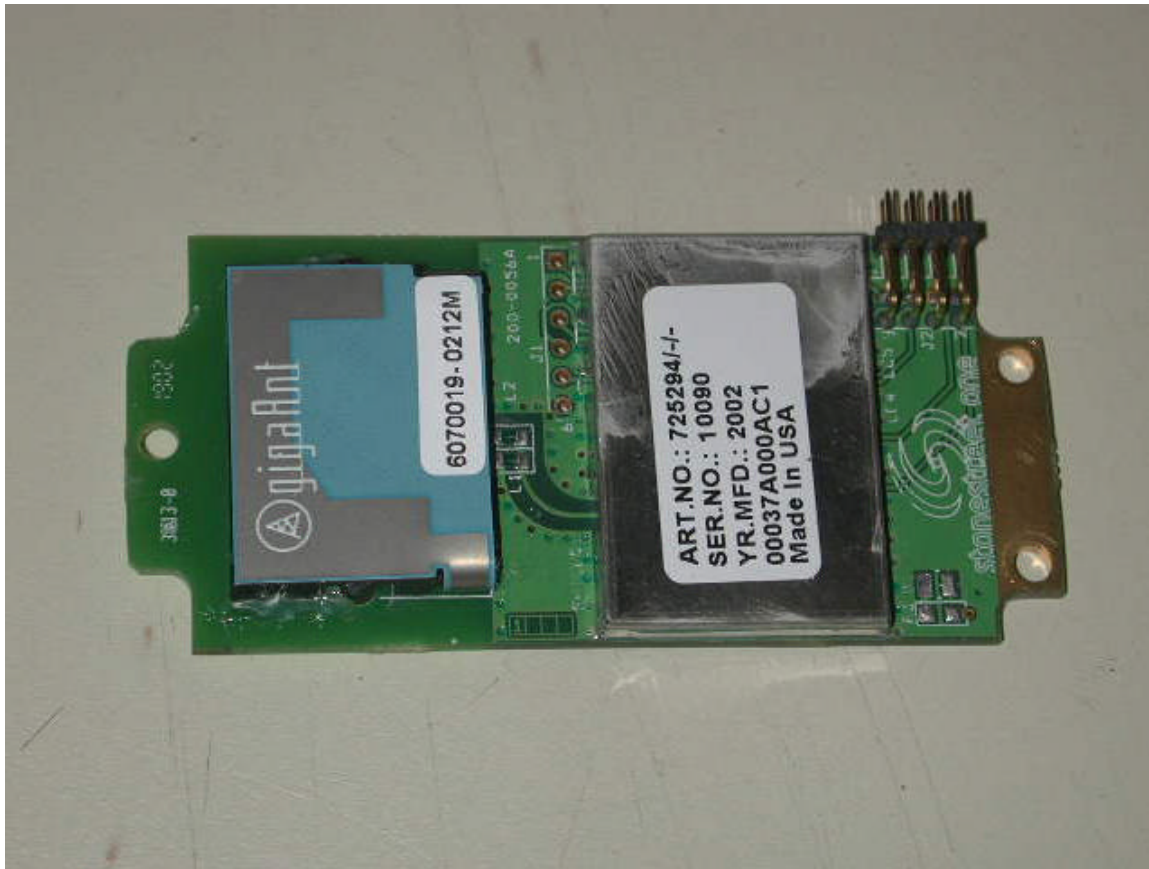
Photo 2 Detail View – Bluetooth module – Top
