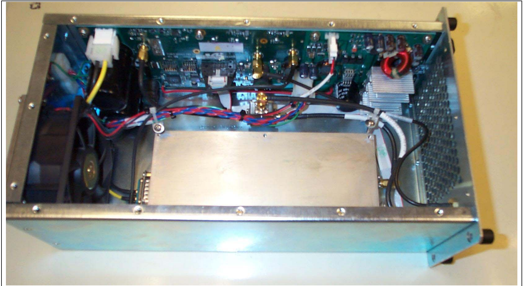
Figure 3. Power Module with power amp heat sink removed, left oblique view.
