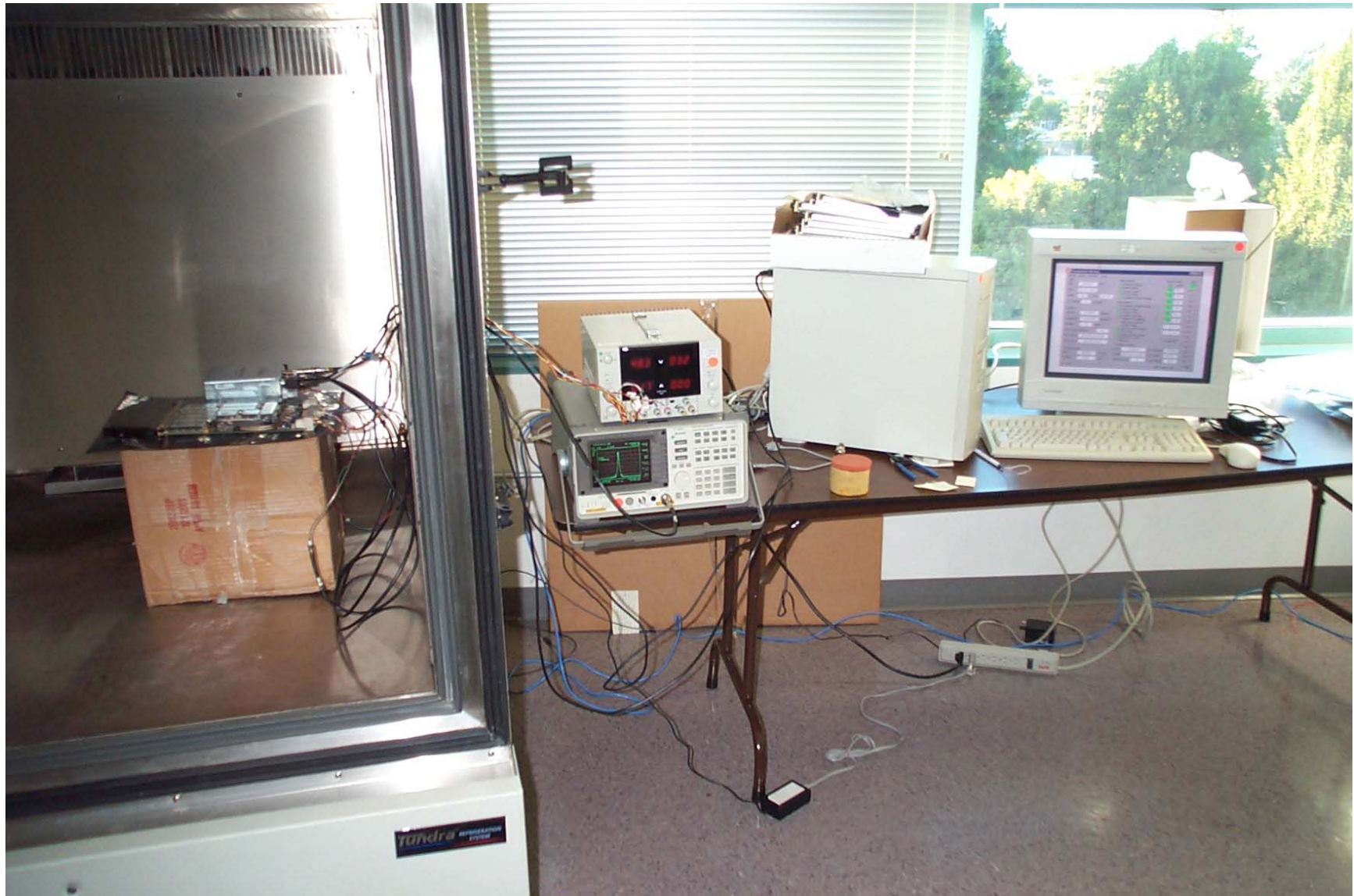
Figure 1. Frequency Stability Test Set-up – Complete View
