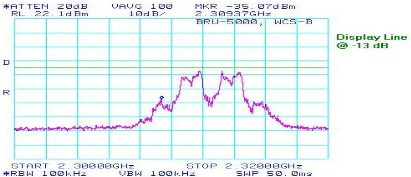
Plot #13: WCSB Spurious Emission 2.3 - 2.32 GHz
