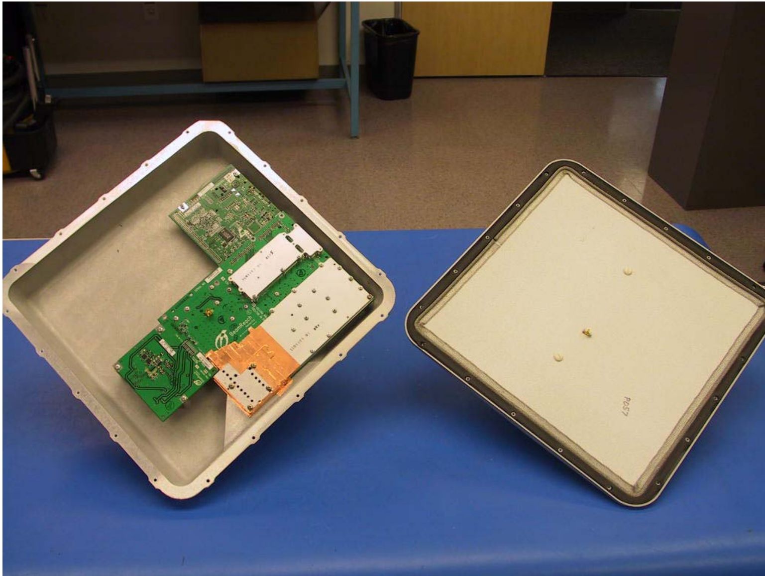
Figure 1. BRU-100 Open View, Electronics on Left, Antenna Ground Plane and EMI Gasket on Right.
