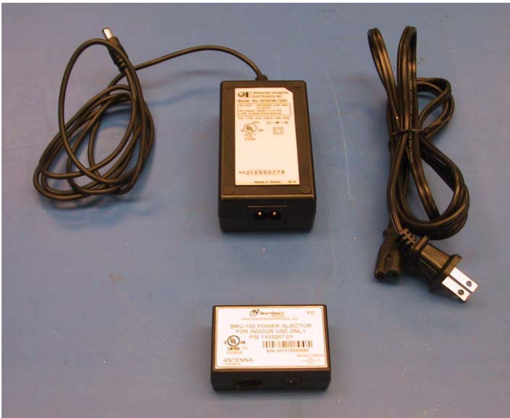
Figure 8. BRU-100 Peripherals, OTE AC/DC Power Supply, Power Supply AC Cord, and Power Injector Module. The Power Injector Provides Interfaces between the BRU-100 Combined Power and Ethernet Cable, The DC Power Supply, and a Standard Ethernet Cable to Customer Computer or Ethernet LAN.
