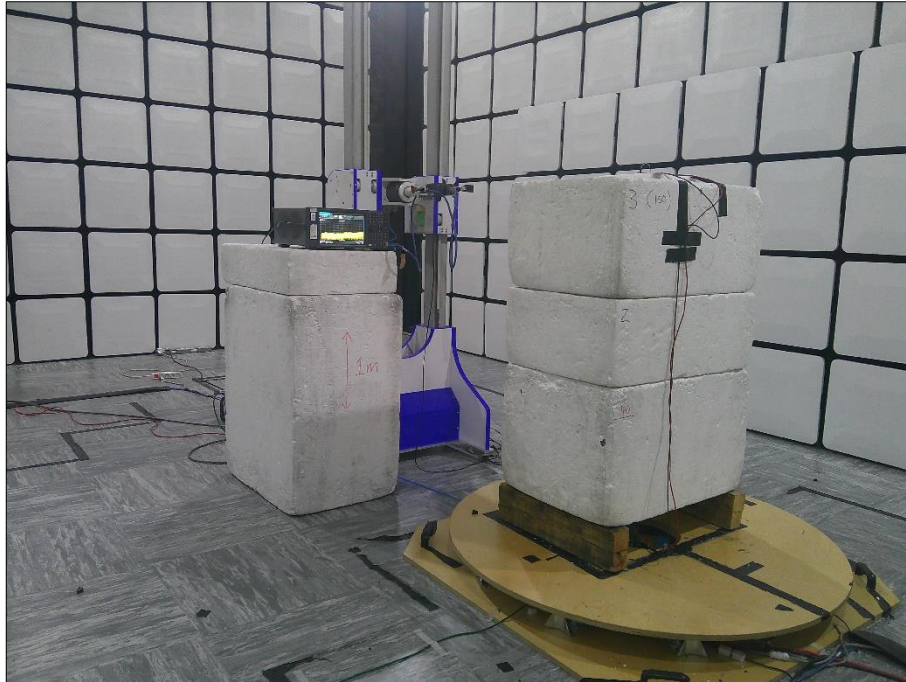
Figure 9 - Test Setup - 18 GHz to 26 GHz
