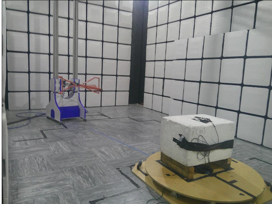
Figure 1 – Radiated Emissions - 30 MHz to 1 GHz (X Plane)
