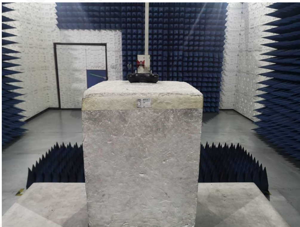
FCC RADIATED EMISSION TEST SETUP ABOVE 1GHZ
