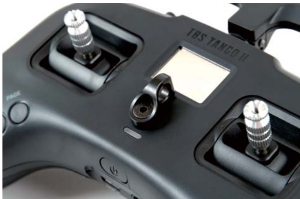
Power button, status LED, neck-strap hook and OLED display
