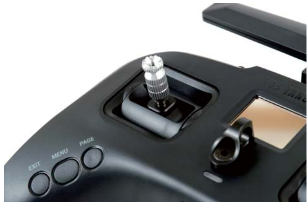
Left gimbal and configuration menu buttons
