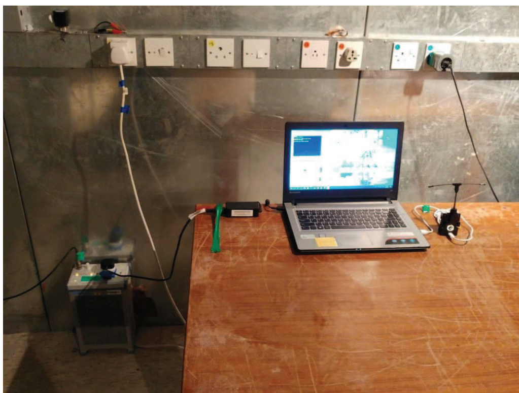
Set-up for AC power line Conducted Emission
