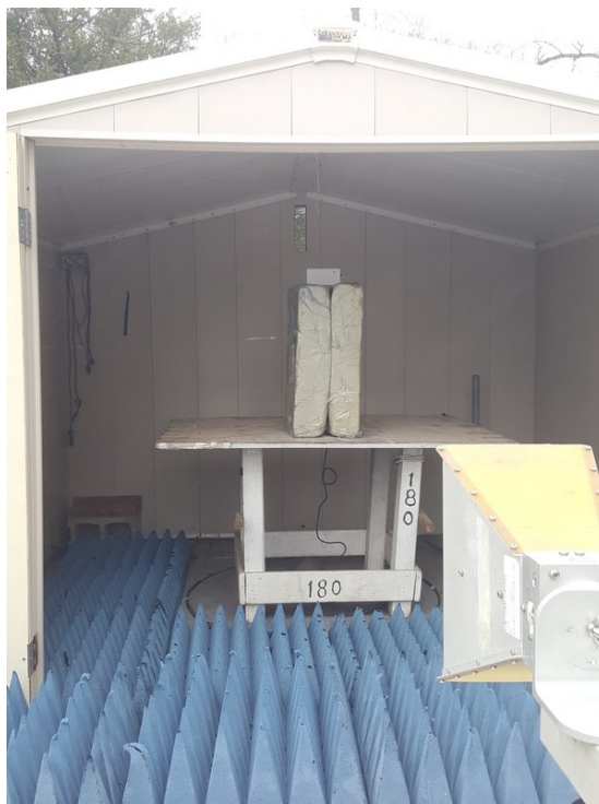
EUT w/ Compact quarter inch ANT pole
