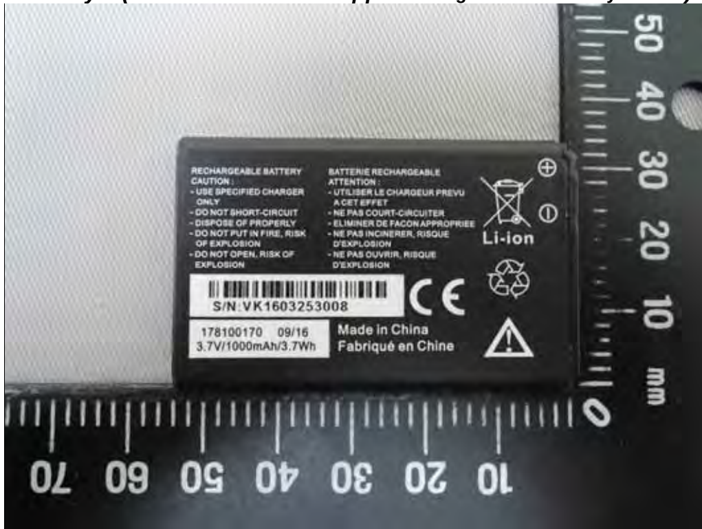
Battery – (Model No.: 5C-1000 Supplier: Ningbo Veken Battery Co.Ltd.)
