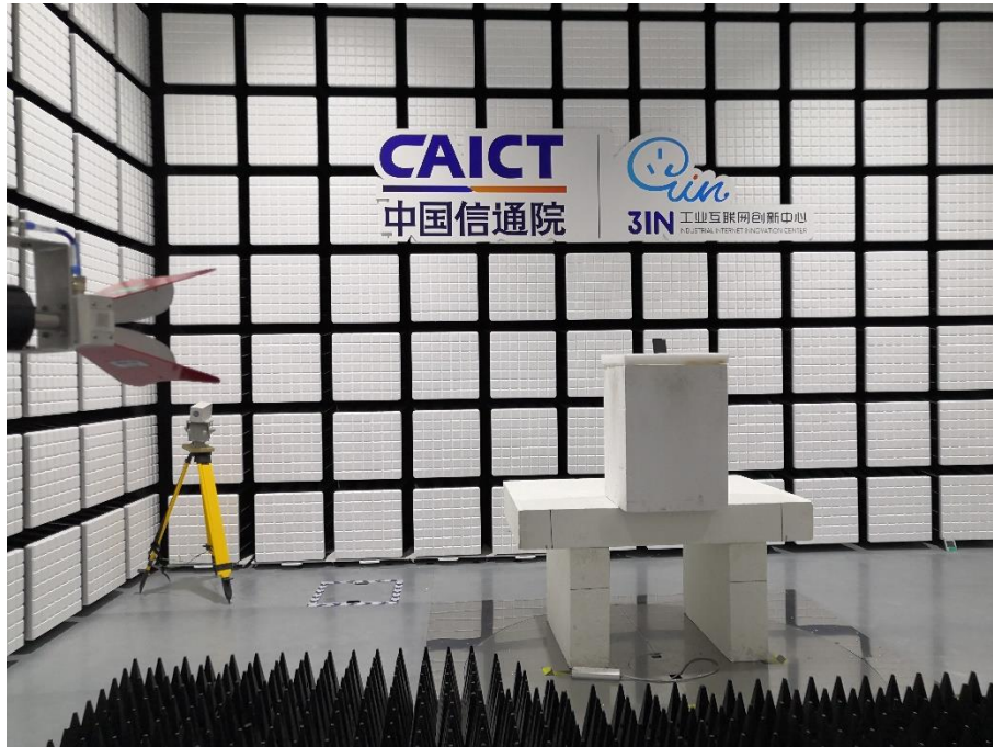
Description: Radiated Emission Test Setup (1GHz -18GHz)
