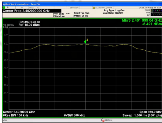
In-Band Reference Level BLE 1M_Channel 0
