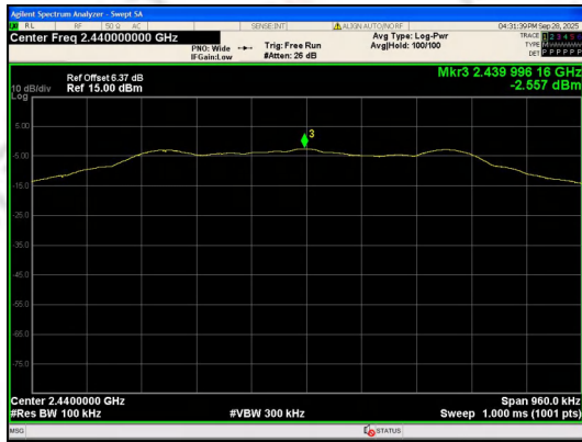
In-Band Reference Level BLE 1M_Channel 19
