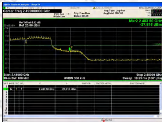
Out Of Band Emission IEEE 802.11n_Channel 9_40MHz_Antenna 0
