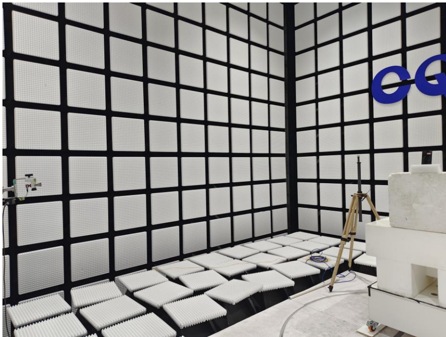
Description: Radiated Emission Test Setup (26.5GHz -40GHz)
