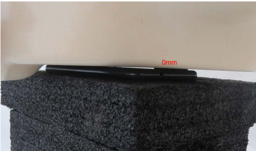
Picture 12: Back Side, the distance from handset to the bottom of the Phantom is 0mm
