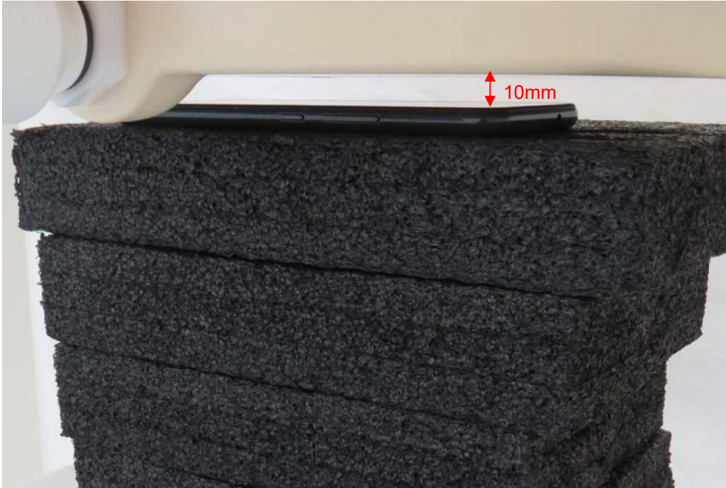
Picture 7: Front Side, the distance from handset to the bottom of the Phantom is 10mm
