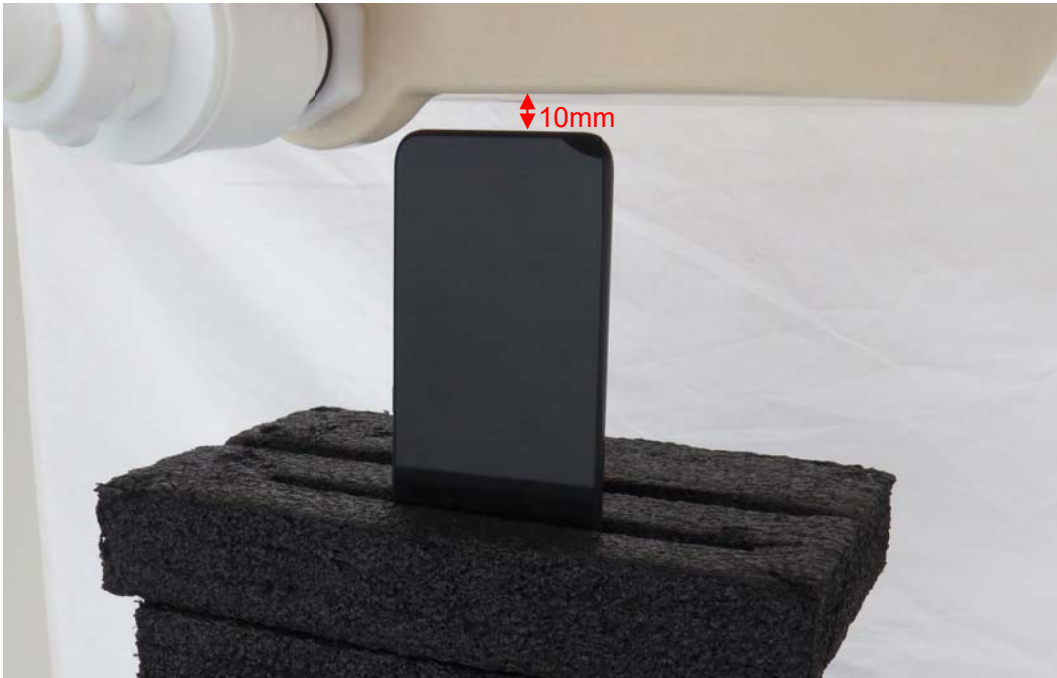
Picture 11: Bottom Edge, the distance from handset to the bottom of the Phantom is 10mm
