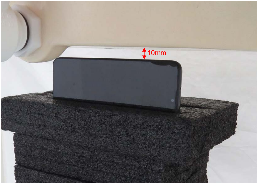
Picture 8: Left Edge, the distance from handset to the bottom of the Phantom is 10mm
