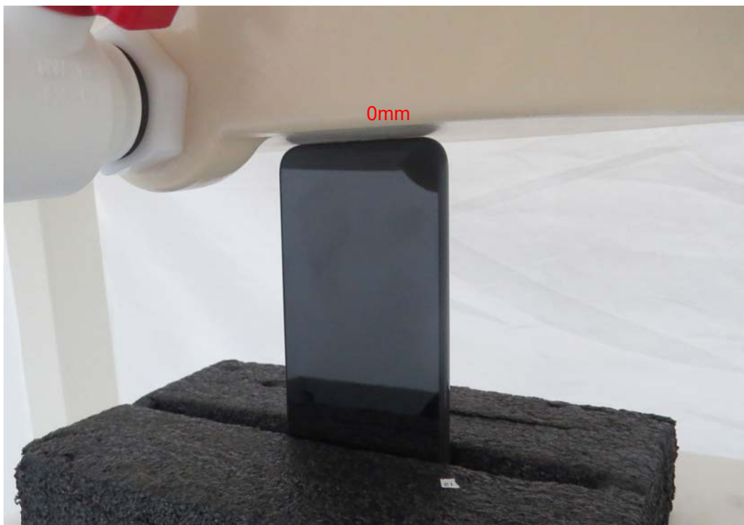
Picture 14: Bottom Edge, the distance from handset to the bottom of the Phantom is 0mm
