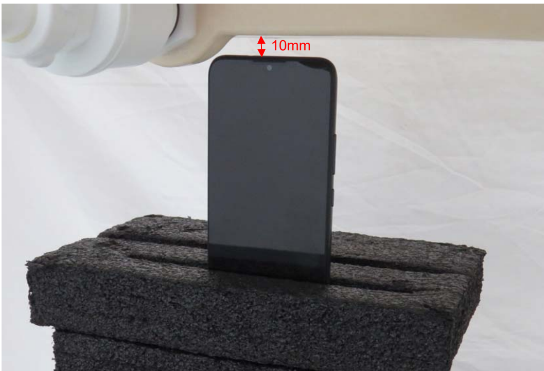
Picture 10: Top Edge, the distance from handset to the bottom of the Phantom is 10mm
