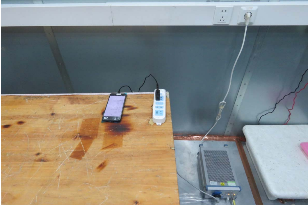
Picture 2 Conducted Emission Test Setup
