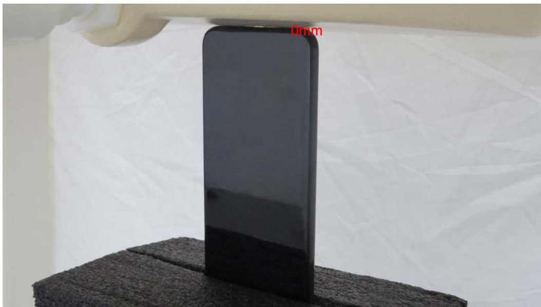
Picture 15: Bottom Edge, the distance from handset to the bottom of the Phantom is 0mm
