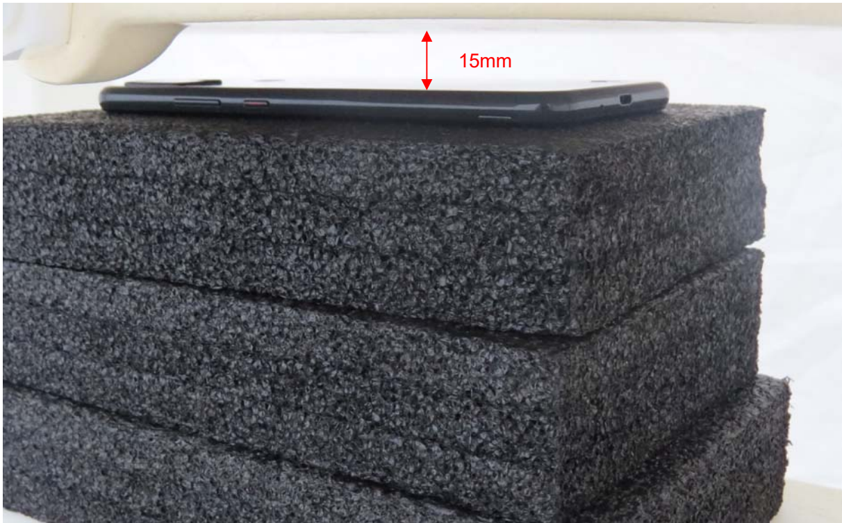
Picture 5: Back Side, the distance from handset to the bottom of the Phantom is 15mm
