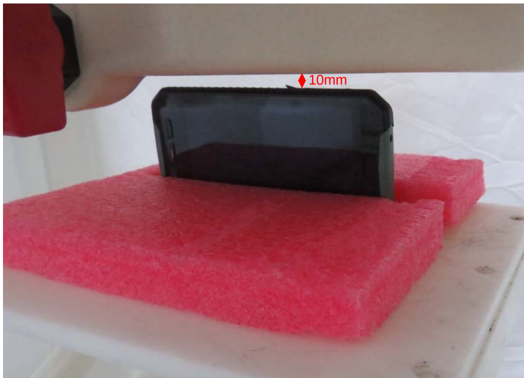
Picture 14: Left Side, the distance from handset to the bottom of the Phantom is 10mm
