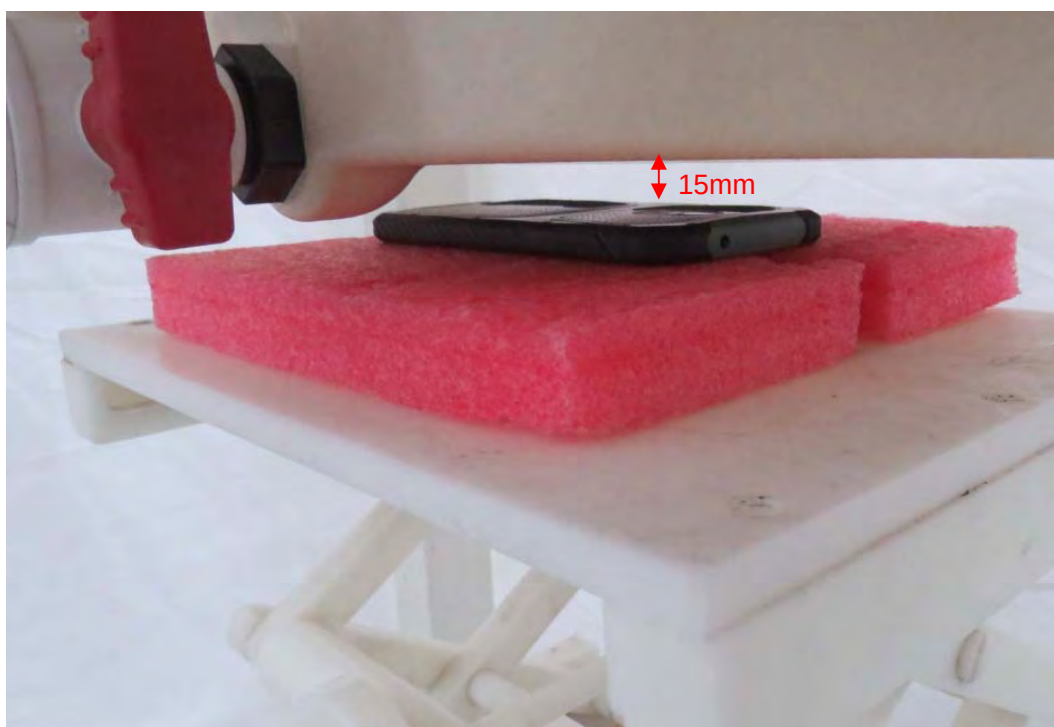
Picture 11: Back Side, the distance from handset to the bottom of the Phantom is 15mm
