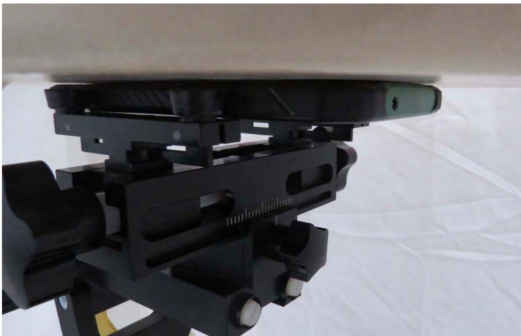
Picture 18: Back Side, the distance from handset to the bottom of the Phantom is 0mm
