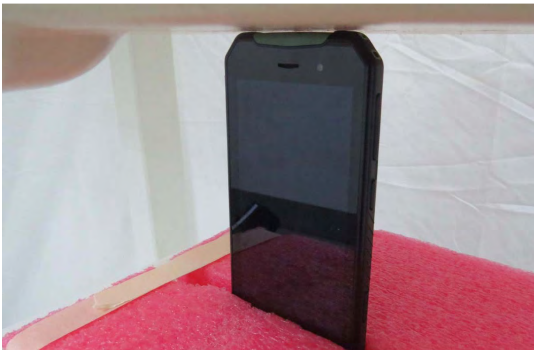
Picture 22: Top Side, the distance from handset to the bottom of the Phantom is 0mm
